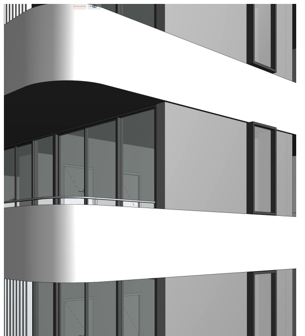
CLD3 Cladding 3_Painted rendered masonry
