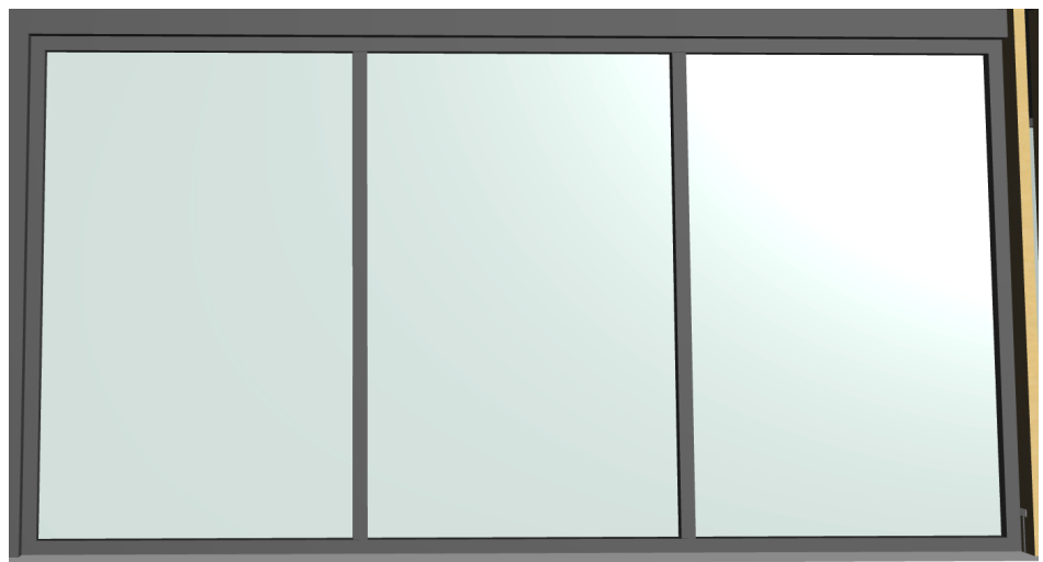
GL1 Glazing 1_Powdercoated aluminium framed clear glazing, PCF2
